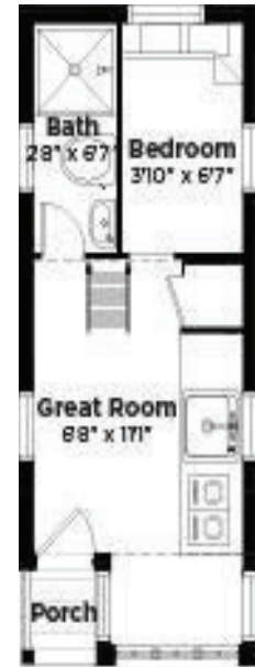
Figure B-1 House with Bedroom and Bathroom Non-Compliant with the OBC. Cypress-Equator, Tumbleweed http://www.tumbleweedhouses.com
